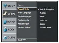
Options to view a picture with a normal (4:3) aspect ratio at 720p or 1080i mode output format.
